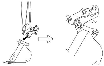
(2) Slowly move the link portion of the Quick Coupler towards the bucket pin to connect.
