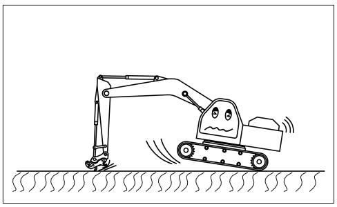
4) Lifting heavy object through quick coupler is very dangerous and may cause the short life span of the quick coupler.
