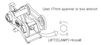
(5) Winch Type of hand-operated Quick Coupler needs to use safety pin or round bar below Ø25 size as below.
