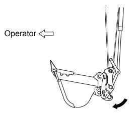
(5) Operate the switch to "Install" position and point the hitch toward the pin of the link side.
