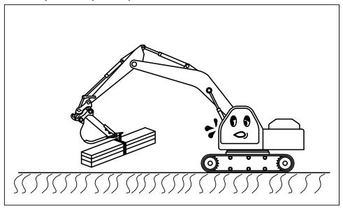
5) In case of installation of a bucket or attachment in reverse direction(face position), high attention is required to keep enough distance(A) to allow entering angle on hook. Please keep this enough distance(A) for correct linkage.
