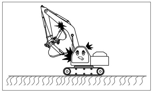
2) Overloaded operation may cause a short life span of quick coupler, attachment and the excavator.
